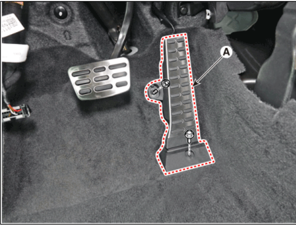
7. Disconnect the accelerator pedal connector (A)
